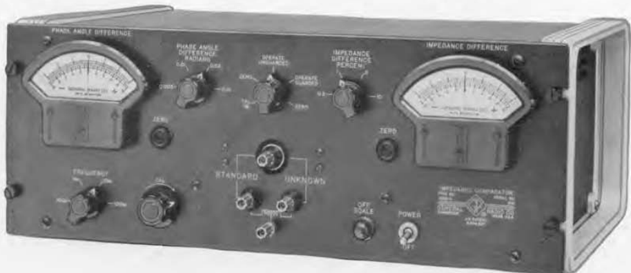
Figure 1. Panel view of the Type 1605-A Impedance Comparator, used for the measurements described in this article.
